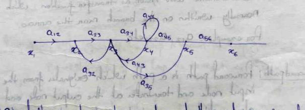
a directed line called branches. Every branch of signal flow graph having an arrow, which represent the flow of signal.
