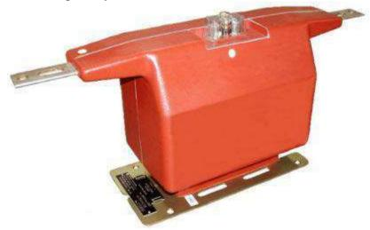
Another very common type of construction is the so-called "window," "through" or donut type current transformer in which the core has an opening through which the conductor carrying the primary load current is passed. This primary conductor constitutes the primary winding of the CT (one pass through the "window" represents a one turn primary), and must be large enough in cross section to carry the maximum current of the load.
